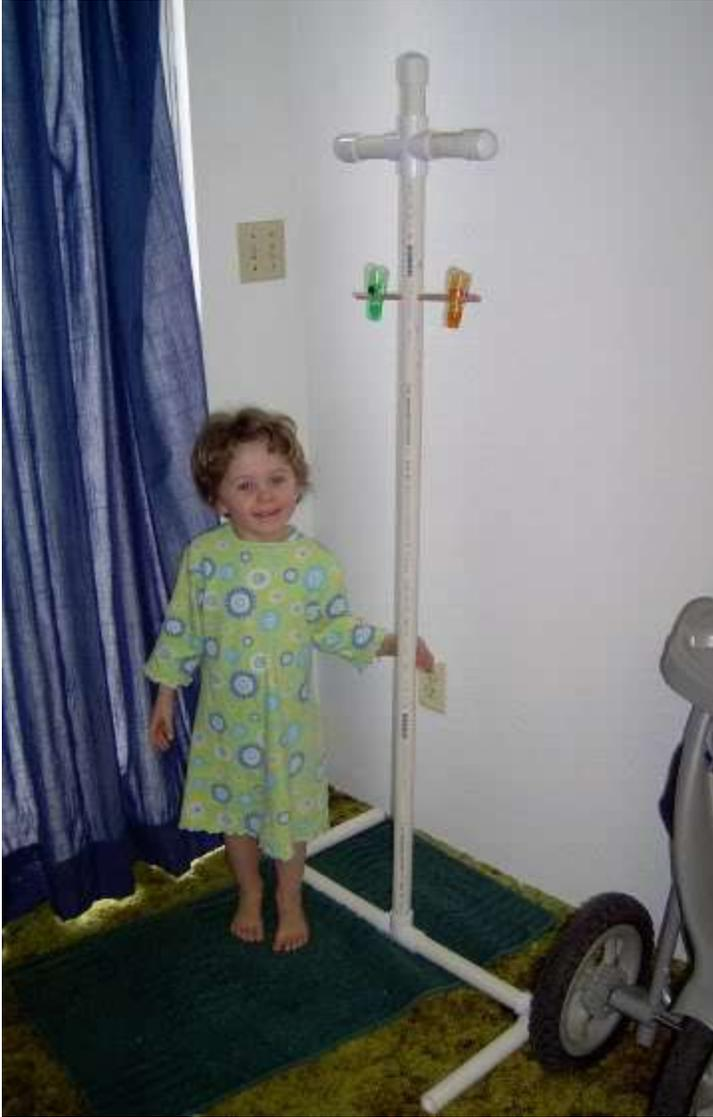
DH went to town with this. He used PVC for the base, with a couple of elbow joints, so he didn't have to figure out how to attach it to a nice board (he said mine is the lazy man's version!) He also drilled holes, so there is a dowel that I can stick through to adjust the height of the pants hangers. And excuse the mismatched dollar store clips, they are now real matching clothespins 😊
