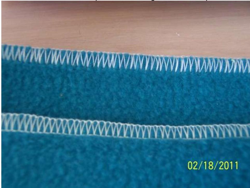
Can you see how it forms V's? That is because the needle thread tension is so loose that the needle thread is being pulled all the way to the edge of the fabric. The bottom line of stitching is just a regular, balanced 3-thread stitch, so you can see the difference.
