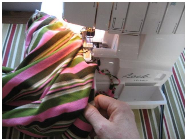
Here the side panel is on the bottom and I'm serging it to the back.
